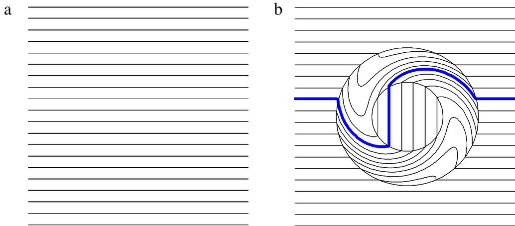
**Fig. 1.** A sketch of transformation method: (a) Initial space with a simple known field distribution; (b) deformed space characterizing the designed function.
