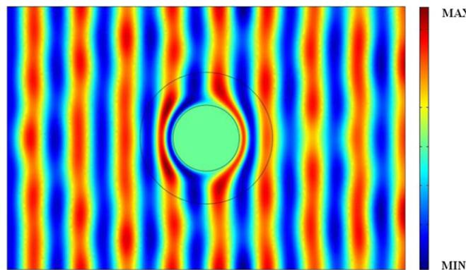
Fig. 4. Simulation of the displacement field around the  $\rho$ -unchanged acoustic cloak.
