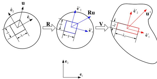
Fig. 2. Rigid rotation and stretch operation during a transformation at each point.
