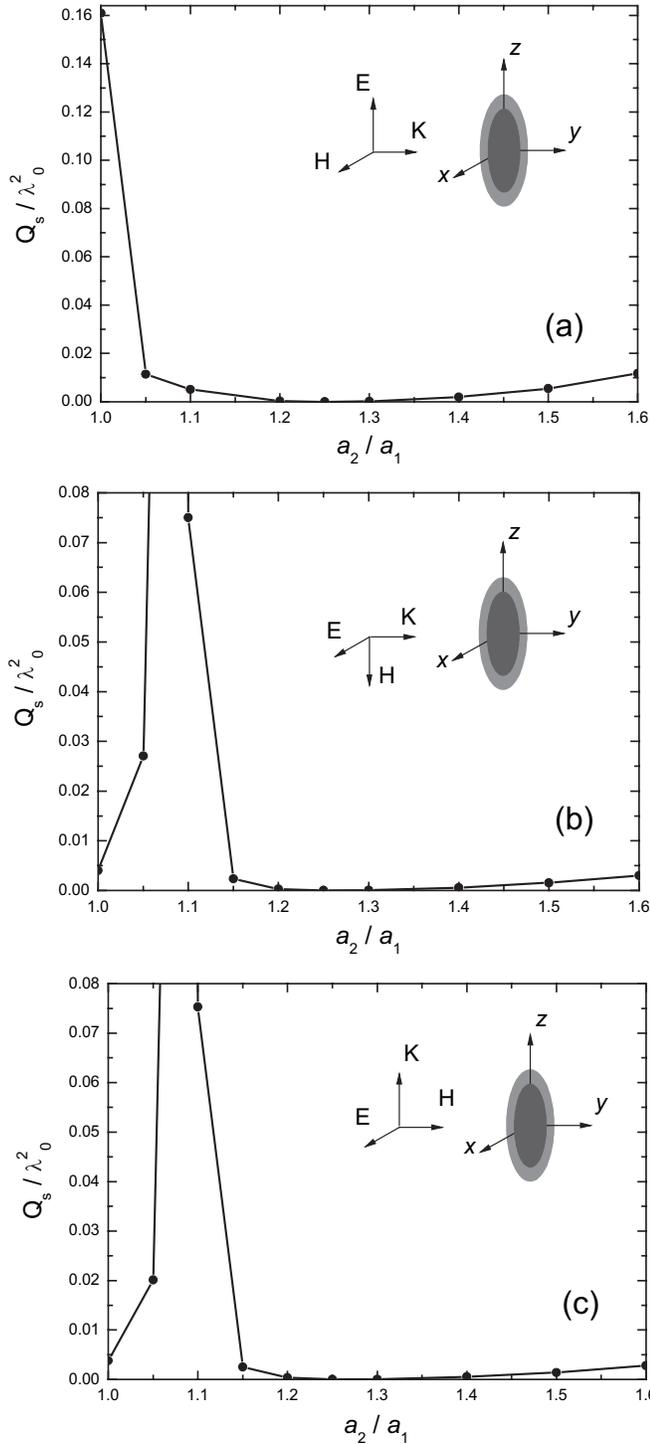
FIG. 8. Normalized total scattering cross section of a coated spheroid vs the ratio  $a_2/a_1$  for three incident cases [ $\bar{\epsilon}_1=(-3, -3, -5.34)$ ,  $\epsilon_2=10$ ,  $\bar{\mu}_1=(1, 1, 1)$ ,  $\mu_2=1$ ,  $\rho=2$ , and  $a_1=\lambda_0/20$ ].
