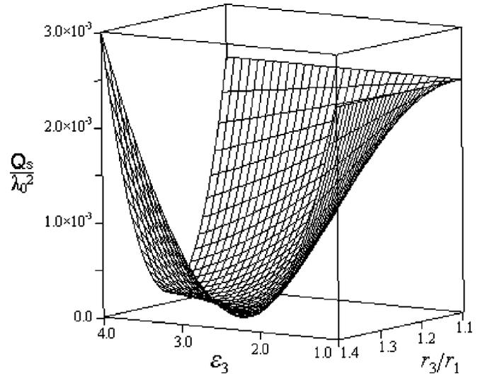
FIG. 6. Normalized total scattering cross section of a doubly coated sphere vs the permittivity  $\epsilon_3$  and ratio  $r_3/r_1$  ( $\epsilon_1=-2$ ,  $\epsilon_2=10$ ,  $\mu_1=\mu_2=1$ ,  $r_1=\lambda_0/10$ , and  $r_2=1.1r_1$ ).
