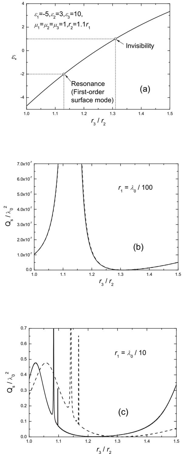
FIG. 4. (a) The effective permittivity  $\epsilon_*$  of a doubly coated sphere assemblage calculated from Eq. (4) and (b,c) normalized scattering cross section of a doubly coated sphere (the solid line) and effective homogeneous sphere (the dashed line) with the permittivity  $\epsilon_*$  and radius  $r_3$ , vs the ratio  $r_3/r_2$  for different  $r_1$ .
