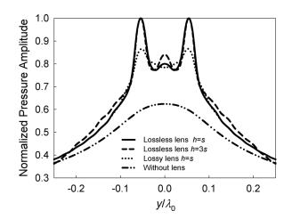
FIG. 4. Normalized pressure amplitudes in the image plane calculated at 1898 Hz in four cases: imaging with the lossless superlens of thickness h = s and h = 3s and with and without the lossy lens of thickness h = s.
