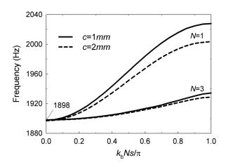
FIG. 2. The dispersion curves given by normalized Bloch wave vector versus frequency for the macro-cell unit of the slab lens with different thickness h = Ns in different separation *c*.
