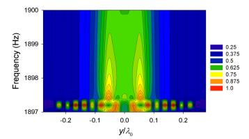
FIG. 3. (Color online) Contour plot of normalized pressure amplitude distributions taken 1 mm behind the slab lens of thickness h=s at different frequencies for two monopole line sources separated by  $\lambda_0/9$  being placed in front of the lens at the distance 1 mm.
